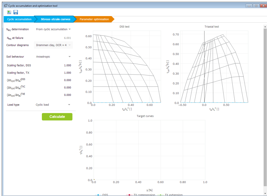
Figure 6.32 Stress-strain curves tabsheet, with contour diagrams for Drammen clay with OCR = 4.
