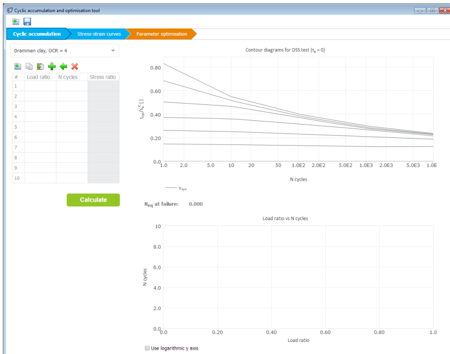
Figure 6.28 Contour diagram for DSS test for Drammen Clay with OCR = 4
