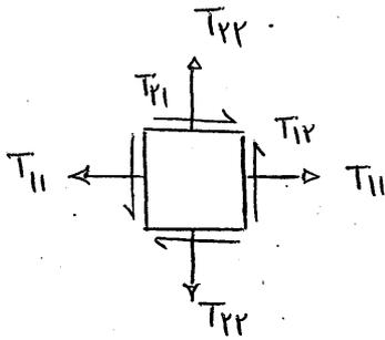
$$T_{ij} = \begin{bmatrix} T_{11} & T_{12} & 0 \\ T_{12} & T_{22} & 0 \\ 0 & 0 & 0 \end{bmatrix}$$
