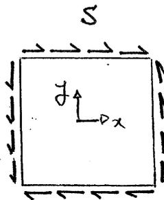
$$T_{xx} = 0, T_{yy} = 0, T_{xy} = S$$
