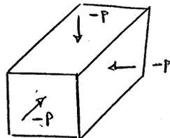
$$T_{11} = -P = \lambda e_{kk} + 2\mu e_{11} = \lambda e_{kk} + 2\mu \times \frac{1}{3} e_{kk} = \left( \lambda + \frac{2\mu}{3} \right) e_{kk}$$
