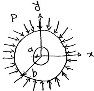
$$U = L \left\{ \underbrace{r^2}_{\text{Suitable}}, \underbrace{\log r}_{\text{unsuitable (multivalued displacement)}} \right\}$$
