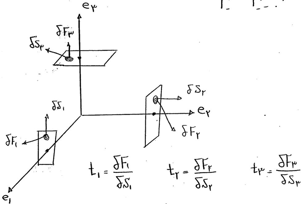
$t_1 =$  traction across to the plane normal to  $e_1$ .
