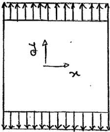
$$T_{xx} = 0, T_{yy} = T, T_{xy} = 0$$
