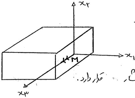
$$T_{11} = Cx_2, T_{22} = T_{33} = T_{12} = T_{13} = T_{23} = 0$$
