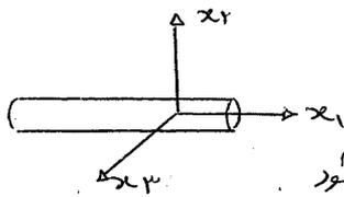
$$T_{11} = \sigma, T_{22} = T_{33} = T_{12} = T_{13} = T_{23} = 0$$
