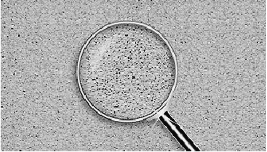
FIGURE 14.1 Close-up view of AAC.
