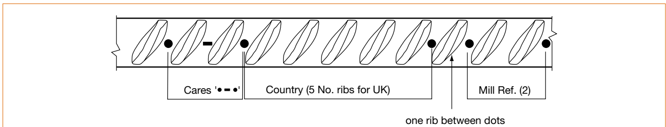
Figure 5.1 Example of manufacturer's identification mark for Grade B500A (using dots)
