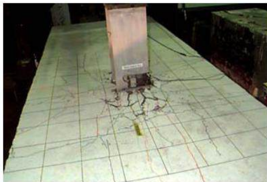
Figure 3.5. Damage to the Floor Slab during Cyclic Rotation of the Column
