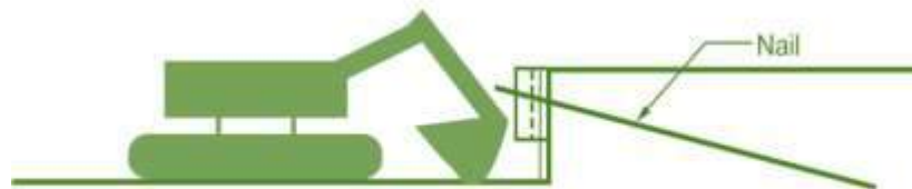
5 Excavation of next lift
