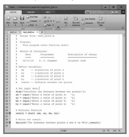
Figure 6.1 M-file test dist2 and function dist2 are loaded into the debugger, with breakpoints set before, during, and after the function call.
