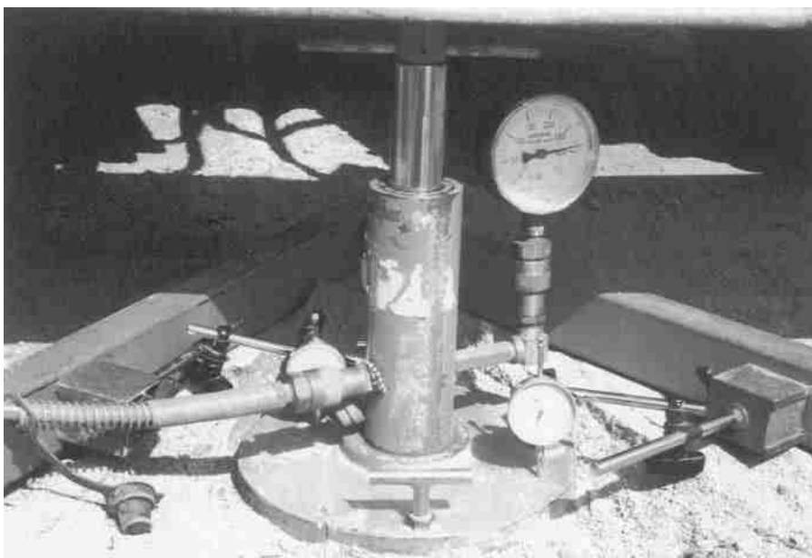
Figure 7.26 Plate load test in the field (Courtesy of Braja M. Das, Henderson, Nevada)
