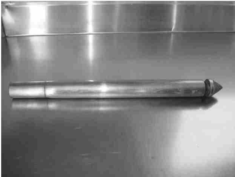
Figure 3.26 Photograph of an electric friction-cone penetrometer (Courtesy of Sanjeev Kumar, Southern Illinois University, Carbondale, Illinois)
