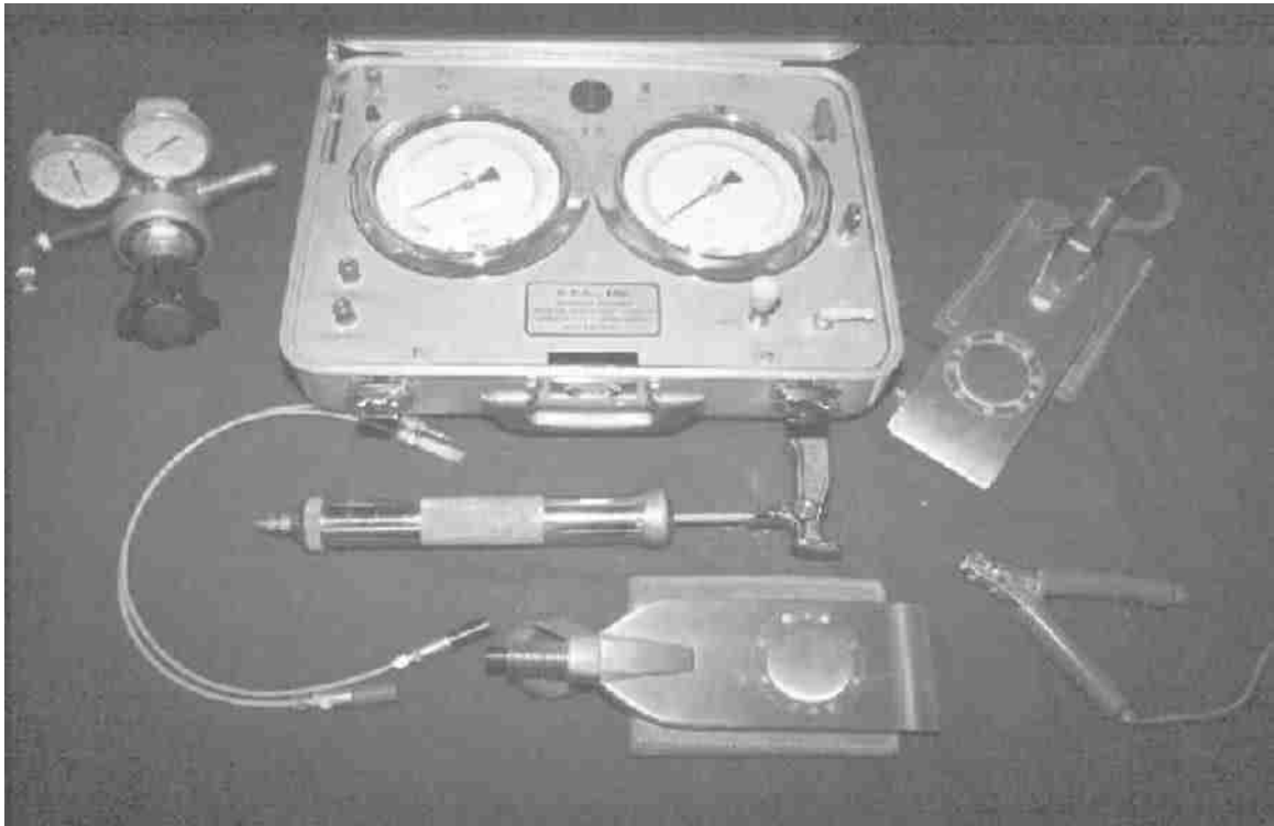
Figure 3.34 Dilatometer and other equipment (Courtesy of N. Sivakugan, James Cook University, Australia)
