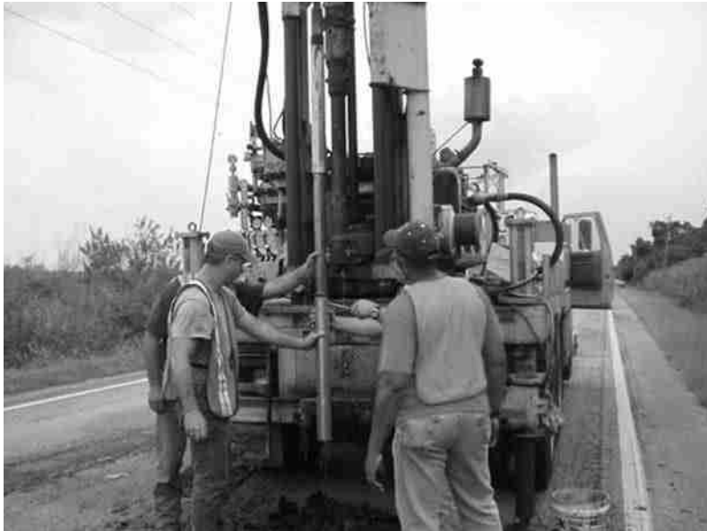
Figure 3.20 (continued) (c) recovery of soil sample (Courtesy of Khaled Sobhan, Florida Atlantic University, Boca Raton, Florida)
