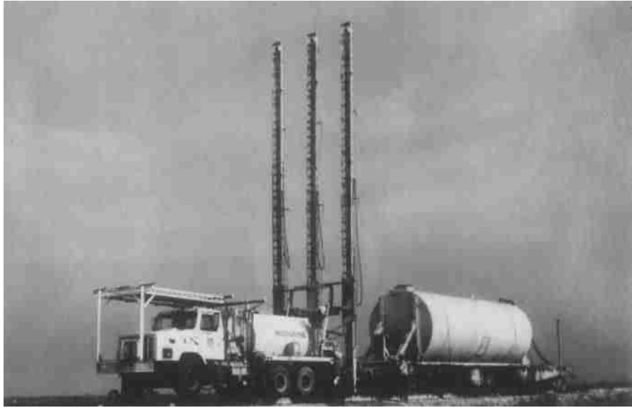
Figure 16.30 Equipment for pressure injection of lime slurry (Courtesy of Hayward Baker Inc., Odenton, Maryland)
