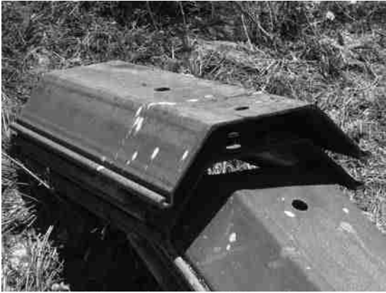
Figure 14.4 Some steel sheet piles at a construction site (Courtesy of N. Sivakugan, James Cook University, Australia)
