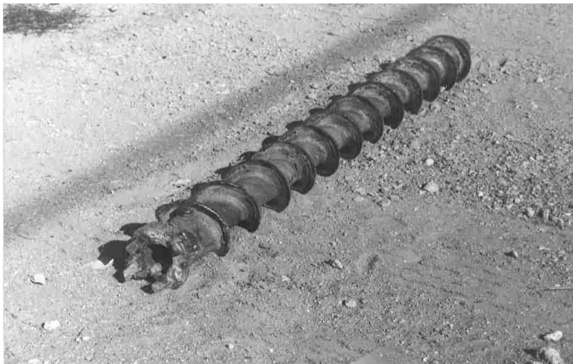
Figure 3.11 Carbide-tipped cutting head on auger flight (Courtesy of Braja M. Das, Henderson, Nevada)
