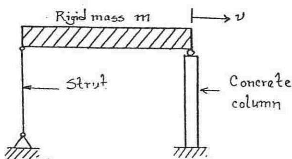
Note that in this model only the column provides the stiffness and the energy dissipation of the system for movements in direction  $v$ . Hence the model and the column have the same properties.
